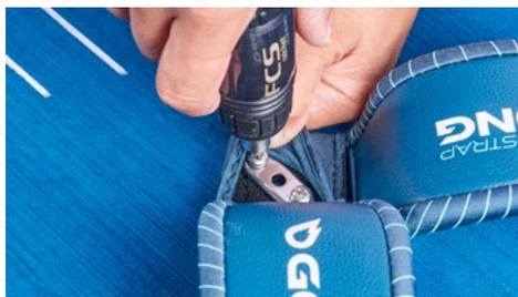
3 **CAUTION:** it is imperative to screw perfectly vertically to the threads and above all not to leave any sand in the threads before screwing. You could cause non-repairable damage to the threads.
